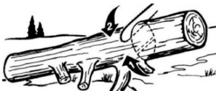
splitting. Then cut from the top. Continue sawing until the two cuts meet. This will prevent the saw from getting pinched.
