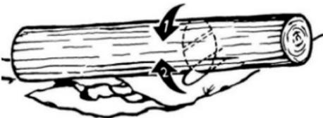
Start sawing from the bottom: cut 1/3 the diameter of the log. This will prevent the log from splitting. Then cut from the top. Continue sawing until the two cuts meet. This will prevent the saw from getting pinched.
